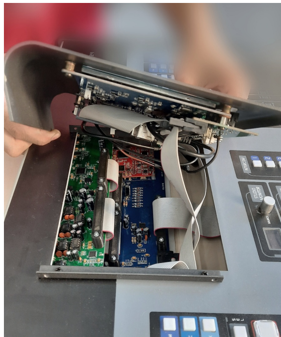
Figure 12: Carefully lift the module to disconnect it
